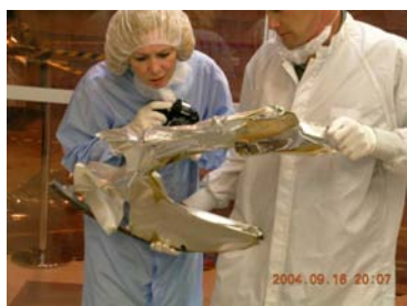
Figure 1. Examination of the 6061 aluminum canister thermal shield in the cleanroom at UTTR.
